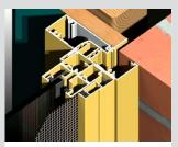
Integrated screening option available. Standard 30mm jamb with built-in nailing fin/weather bar into brick veneer wall illustrated above.
